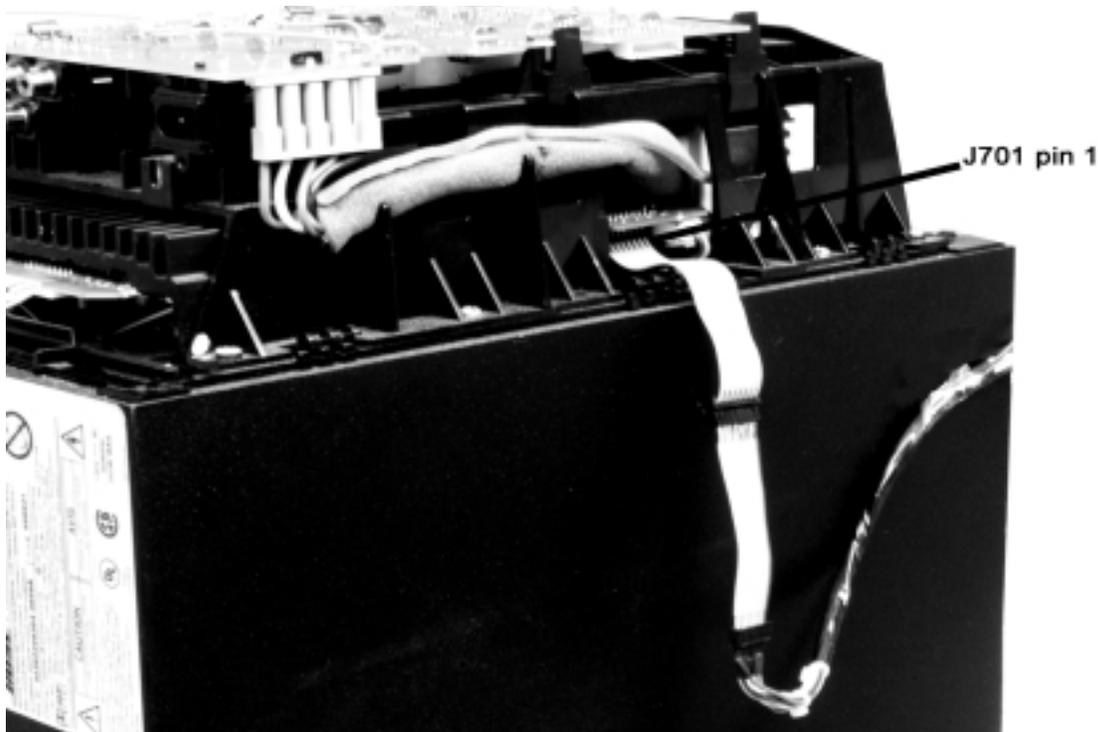
Figure 3. Output Wire Connection View at J701
